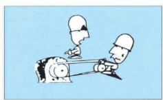
Slack off on take -up until belts can be placed in grooves without forcing.
