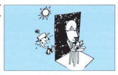
Do not expose belts direct to sunlight during storage. Store belts in shelves or hang belts on racks. Avoid placing belts on floor or ground Avoid piling belts up. Avoid storing belts in heavily bent condition.
