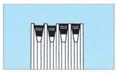
Make sure all pulley grooves are equal in dimensions.
