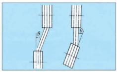
Check pulley alignment. Misalignment of pulley will shorten the belt life. Keep deflection angle less than 1/3°.
