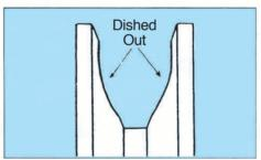
Check pulley for groove wear. If more than 1/32 inch (0.794mm) of "Dished Out" can be seen, short belt life may be expected.
